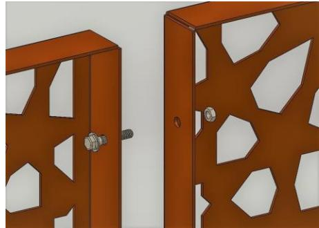
Frameless panels utilise the sheet itself to create a fully integrated and cost effective framing system. With double returns on all four sides, the panel is strong enough to work as both a fixed and sliding screen.
